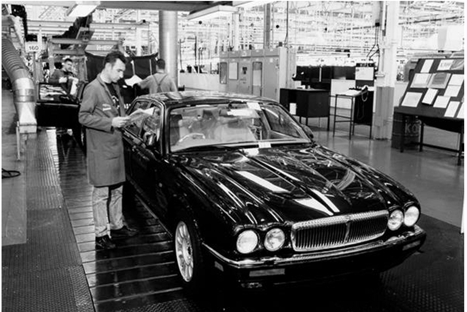
Jaguar's Browns Lane production line. Here a Daimler Double-Six XJ X300 is receiving its final check prior to distribution.
