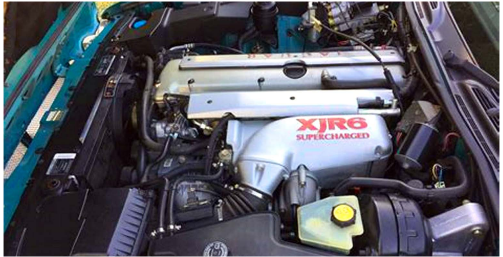
1995 XJR supercharged AJ16 engine producing 326 hp (243 kW; 331 PS) and 378 lb-ft (512 N-m) with the use of an Eaton M90 supercharger and an air-water intercooler.
