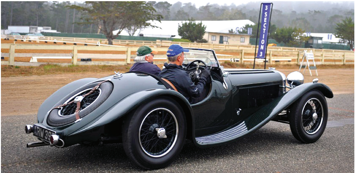
S.S. 90 Prototype showing the distinctive sculpted rear tail treatment. The factory decided that the complex sculpting was too expensive and time consuming and the production cars incorporated a more practical - squared-off rear deck. The Prototype was restored in the USA (Arizona) where it was a Multiple Pebble Beach Concours Award Winner before returning to its owner in Switzerland. The car was recently sold in the UK for an undisclosed amount.
