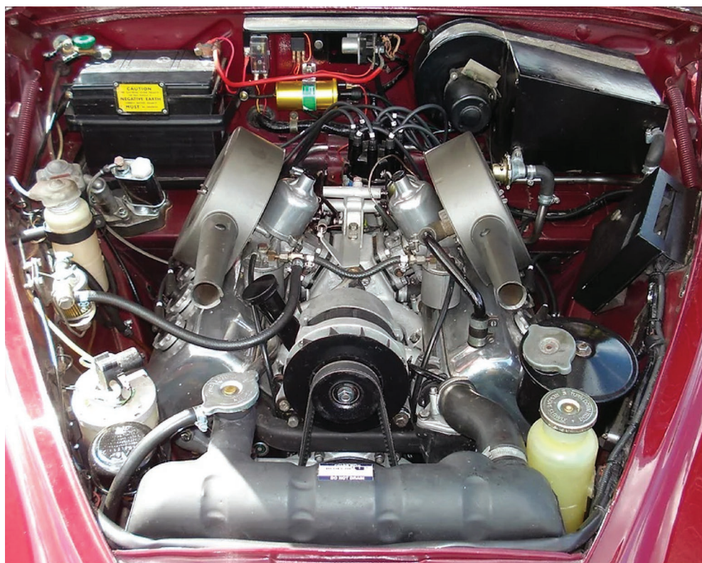
Engine bay of the updated 1967-1969 Daimler V8-250 fitted with an alternator instead of a generator and twin air cleaners, one for each carburettor.
