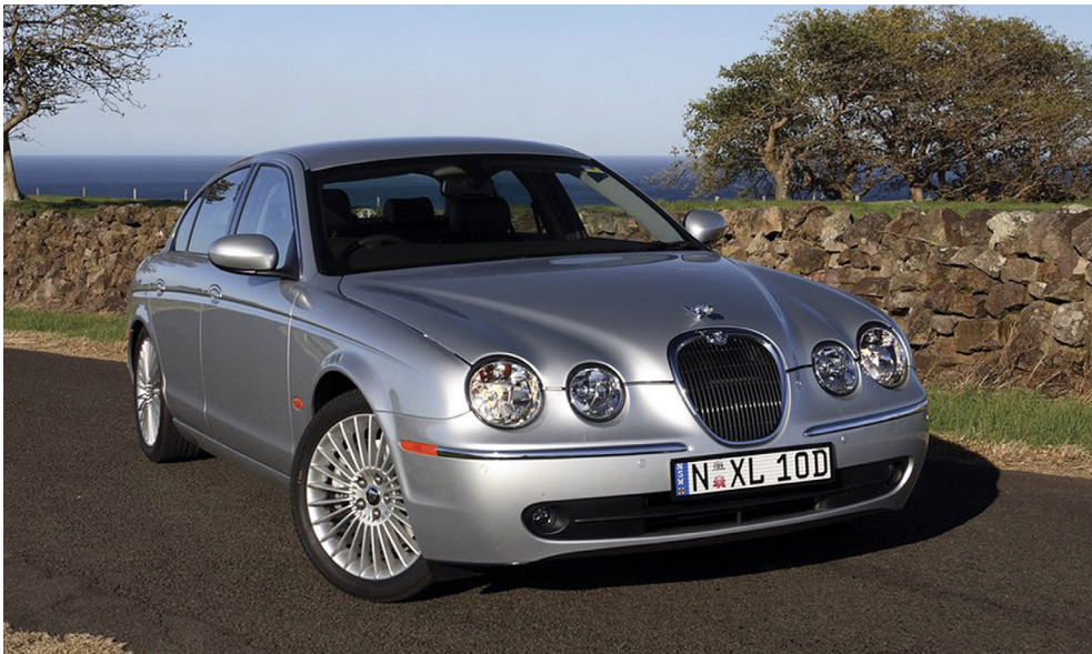
The 2006 X206 S-Type introduced a 2.7-litre twin-turbo-diesel V6 engine. The X206 S-Type could be identified by its bonnet-mounted 'leaper' and new tail-lights.
