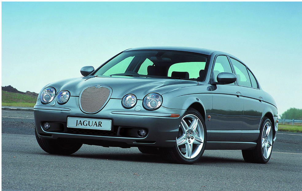
The X202 introduced new engines and ZF transmissions, a stronger chassis, additional safety equipment and greater refinement and an additional model (S-Type R). Visually, the S-Type R (as shown above) can be identified by its bright-finish mesh grille.
