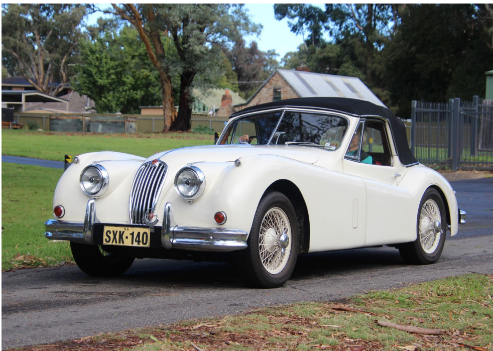
Peter Goodale, 1956 Old English White XK140 (DHC) (80.7110) The car was fully restored 1999-2001 and fitted with front disc brakes, 4.2L engine and 5-speed gearbox. More recently fitted with period wire wheels & electric power steering.
