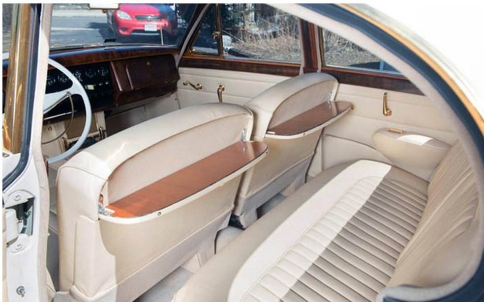
Every piece of internal chrome work was re-plated in gold to match the 'Golden' 3.8 Mk II.
