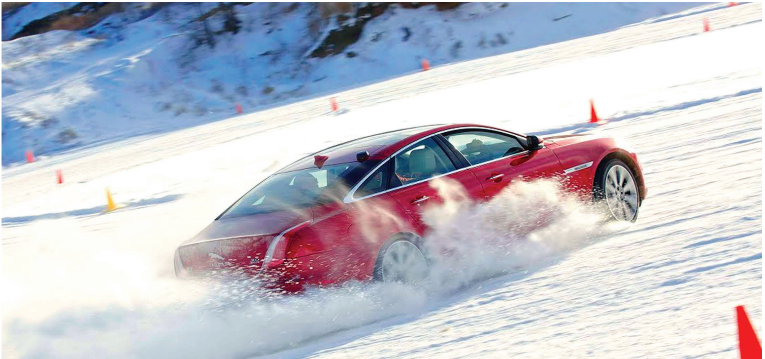
Jaguar Ice Driving Experience. In 2013, the X351 became the only XJ equipped with all-wheel drive. With the increased capability, the AWD's were made available for owners who lived in regions where snow and ice made winter driving hazardous, notably the US Northeast and Midwest, and Canada. The all-wheel drive cars were only available with the supercharged 3.0 litre V6 petrol engine.
