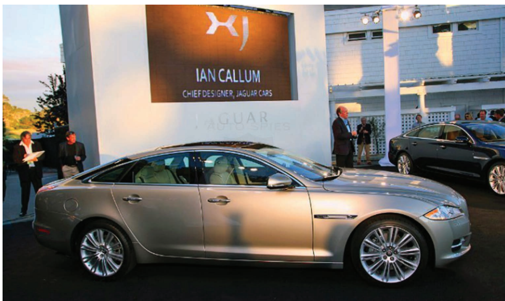
In the US, the XJ was unveiled at the 2009 Pebble Beach Concours d'Elegance. Like the X350, the X351 had a monocoque structure made from aluminium alloy components riveting and bonded together with aerospace-based processes. The car was 50kg lighter than the smaller XF.
