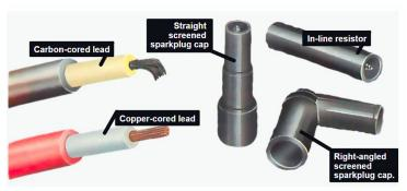
Take care that the combined resistance of HT suppressors in the coil lead, distributor plug leads and plug caps does not exceed 25K Ohm. Otherwise, ignition power could be reduced.
