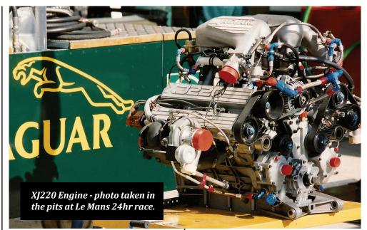
with twin overhead camshafts and four valves per cylinder. Added to the lightweight unit were two Garrett turbochargers.
