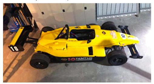
The car has no alternator or thermo fan in order to save weight and not sap engine power. I plan to add a thermo fan (which would only weigh the same as a Mallala hamburger) so as to aid cooling when slowly driving back to the garage at the end of a race.
