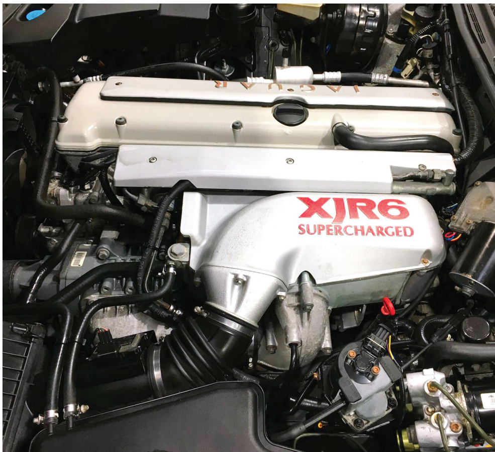
AJ16S. A supercharged version of the 4.0 litre AJ16 was released in 1994 in the X300 XJR6 which used an Eaton M90 blower to boost output to 322hp and 378 lb-ft)
