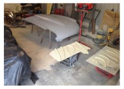
I also had to make new rolled edges for both of the front fenders as they were rusted away. Once the bonnet was fitted, I then pulled the car apart and sprayed the inside and undersides of doors, bonnet and rear hatch.
