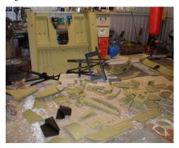
Each after-market panel had to be tech screwed in place first before welding. This is because I found most of the panels didn't fit properly and had to be slightly modified.
