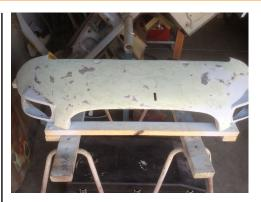
It took about six months to get it right and make it fit properly. I used strips of lead and made patterns from the good side of the bonnet. I then used these to get the shape correct on the damaged side. With a lot of cutting, hammering and shrinking it came up better than expected.
