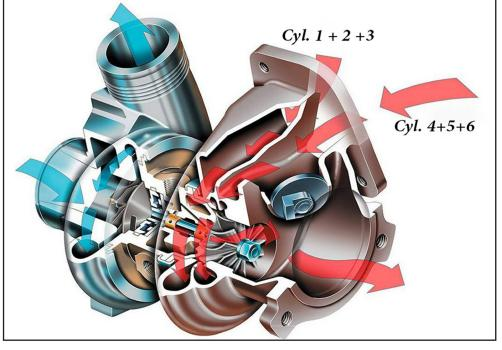
Twin scroll turbo's offer several benefits including taking up less space than a comparable twin turbo system, they provide a faster boost response and better fuel consumption (up to 5%). The above diagram is for a six cylinder engine - firing order 1,5,3,6,2,4.
