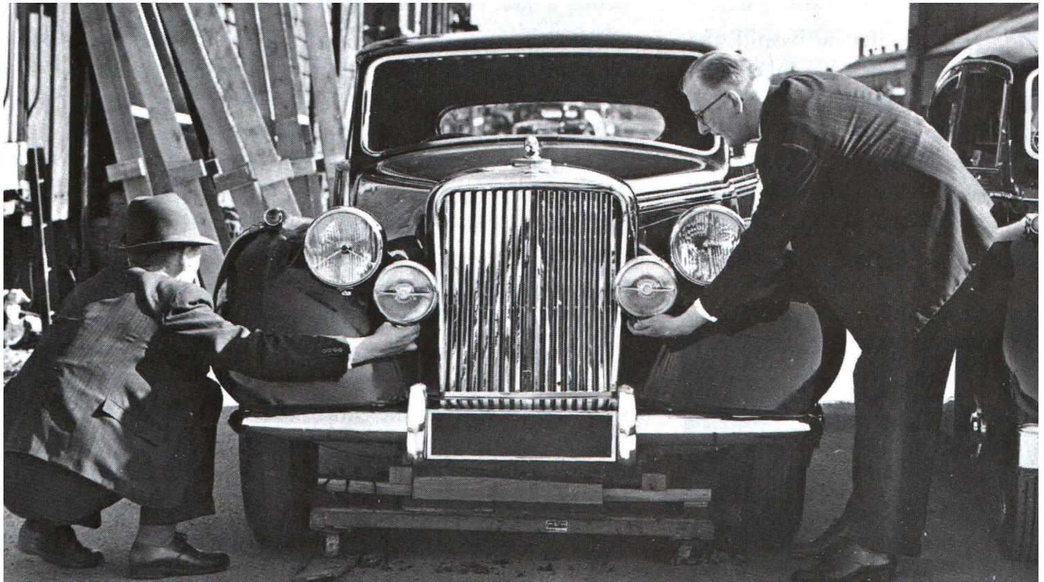
Fred Gardner (Lyons' styling "interpreter") and Lyons working on a Mk V mock-up to arrive at the ultimate position of the auxiliary lights
