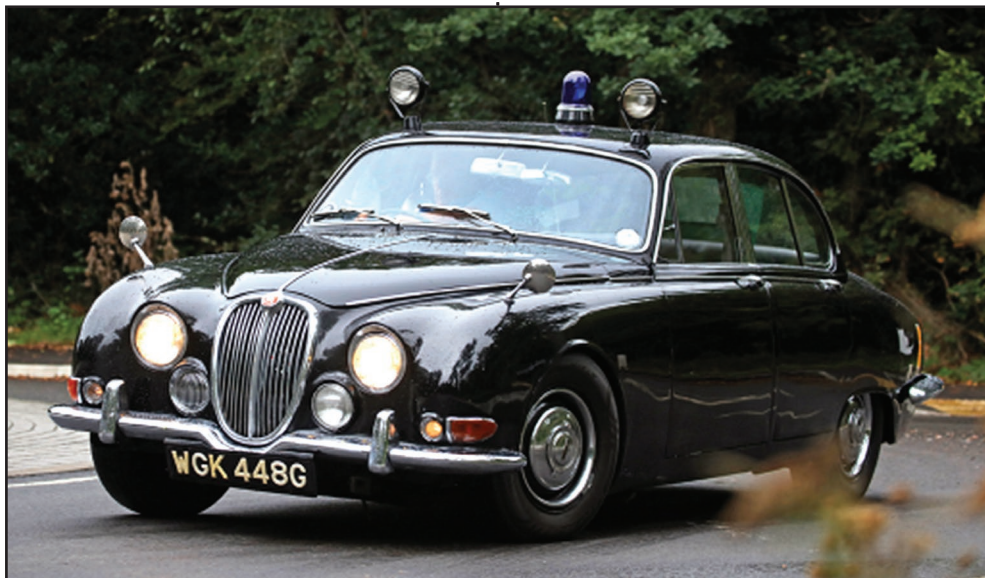
The Black 'S' Type area cars used Auto transmissions with no Park or Low able to be selected.
