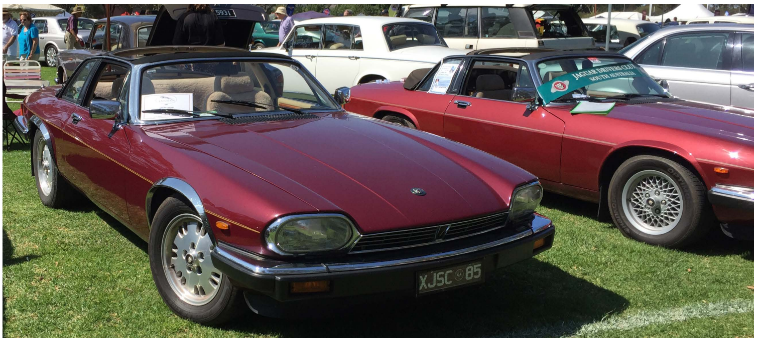
Timothy Telfer 1985 3.6 litre XJ-SC Cabriolet (left) and Rodney Lovell 1986 5.3 litre XJ-SC Cabriolet. Instead of the complicated bracing required to convert the Coupe into a Convertible, rigidity in the Cabriolet was retained by using a central structural bracing hoop over the driver and passenger. The Cabriolet design was a clever low-tech solution.
