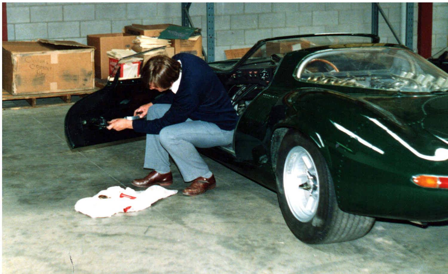
Steve in the Custom's shed carrying out repairs to the damaged door on the XJ13
