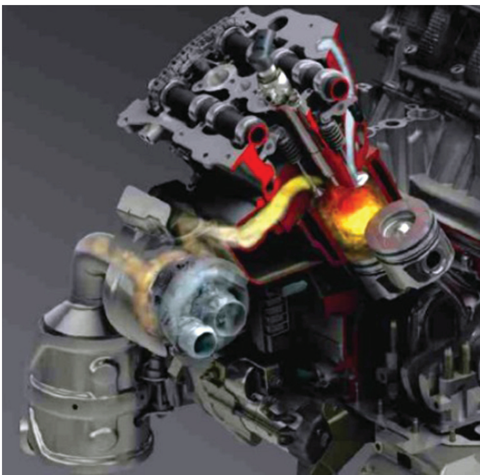
This view illustrates the gas flow, from the long inlet tract, through the cylinder and short exhaust tract to the turbocharger and close-coupled catalyst, where any unburned fuel is turned into CO 2 and water.
