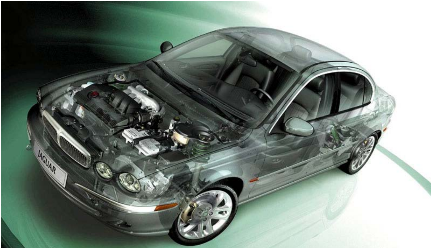
The X-Type at launch was solely a four-wheel drive car. The design brief imposed meant that the X-Type had to feel like any other Jaguar. The only reasonable way to achieve that was with a rear biased all-wheel-drive set up. The car was powered by (more-or-less) the same V6 as installed in the mid-size S-Type that would go on to power future XJ's and the XF.
