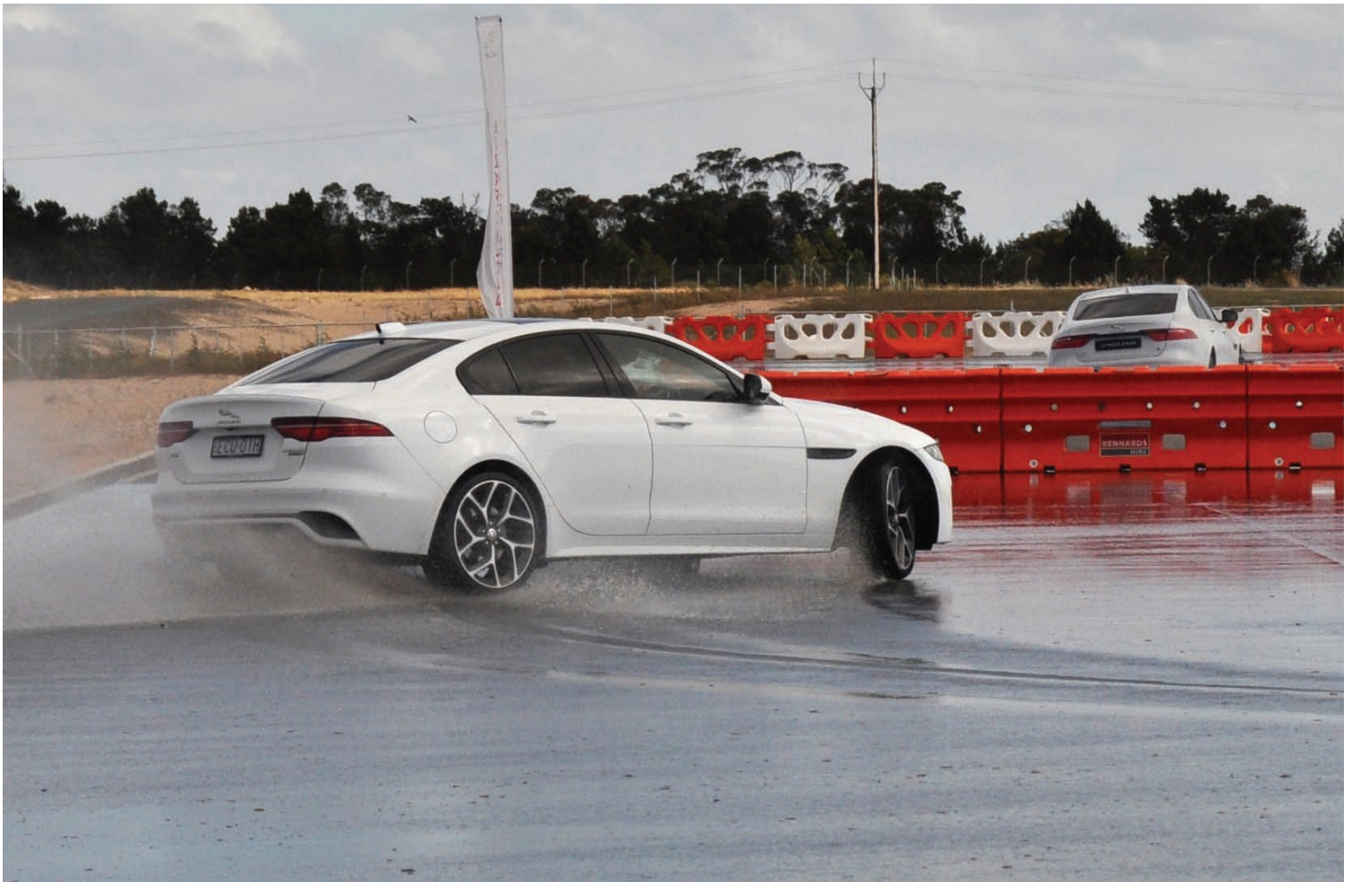
Turbocharged XE on the skid pans showing the benefit of traction control.
