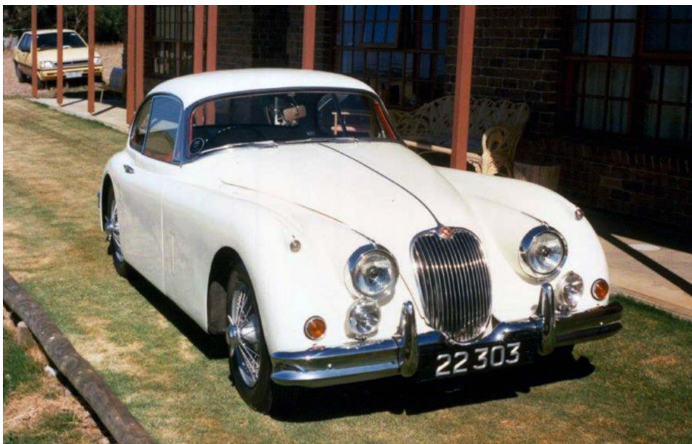
Onslow & Wendy Billinghamurst, 1958 3.8 Litre XK150 (FHC). The XK150 can be easily identified from its predecessor (XK140) by the one-piece wraparound windscreen, less pronounced wing line and a fuller rendition of the grille combining to give the new model a more modern appearance without losing the feline grace common to all Sir Williams' Jaguars.
